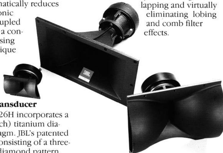
The horn contours were computer-designed to yield smooth response, low distortion, and even coverage. This design avoids the performance disadvantages of horns that utilize sharp flare transitions and flat sidewalls. The Bi-Radial compound flare configuration provides constant coverage over defined, solid angles. To ensure lightweight, superior strength, and freedom from resonances, the horn bell is constructed of molded structural foam.
