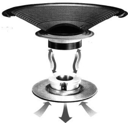
As a voice coil's temperature rises, so does its impedance, causing power compression. Every dB of increase impedance translates into one less dB of output. JBL's exclusive Vented Gap Cooling™ pumps air through the gap and directly over the voice coil to provide immediate heat transfer and reduced operating temperatures, which in turn reduces power compression. VGC technology delivers twice the power handling and gives you greater output by controlling power compression.
